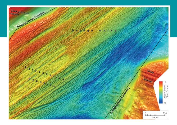
Seabed monitoring data for aggregate extraction area 351, 12 km east of the Isle of Wight, showing the results of a high resolution bathymetric survey over dredged seabed. There are over three million data points spaced just 0.5 metres apart recording water depths within the area shown. Criss-
