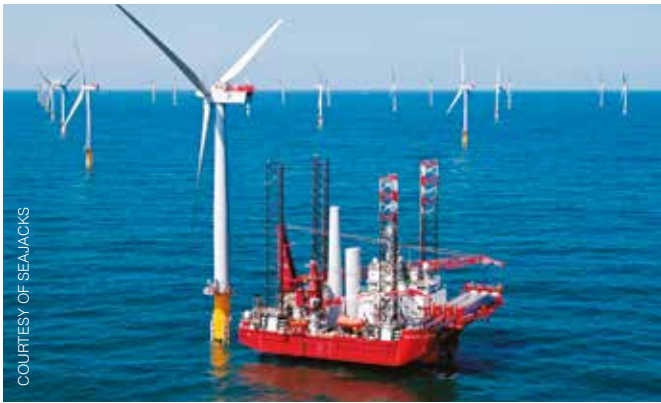
Figure 9: Examples of jack-up vessels used in the O&M phase of offshore windfarms
