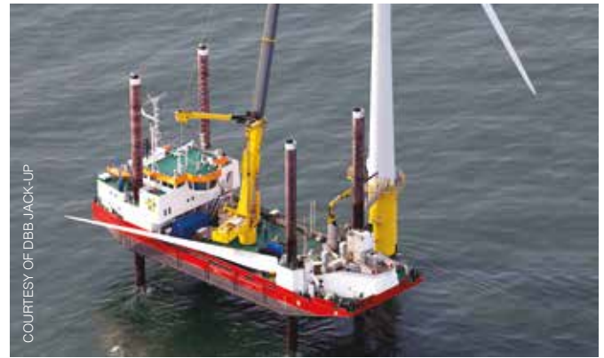
Figure 9: Examples of jack-up vessels used in the O&M phase of offshore windfarms
