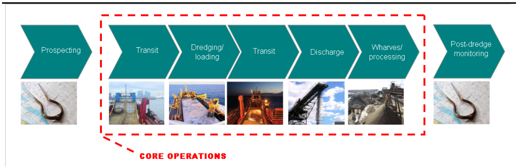
Figure 2.2 Process map and boundaries for calculating a cradle to gate carbon footprint for marine aggregates*
