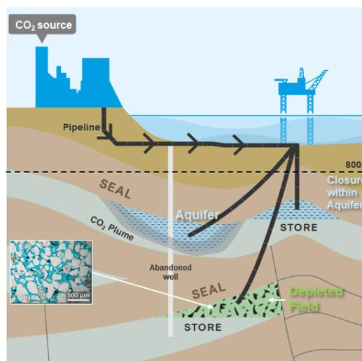
Figure 4.16: Typical CCUS Project Schematic
