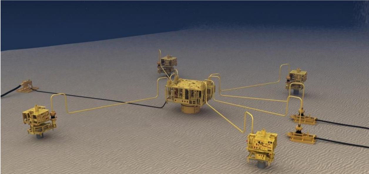
*Figure 4.17: Typical Subsea Manifold and Wells*
