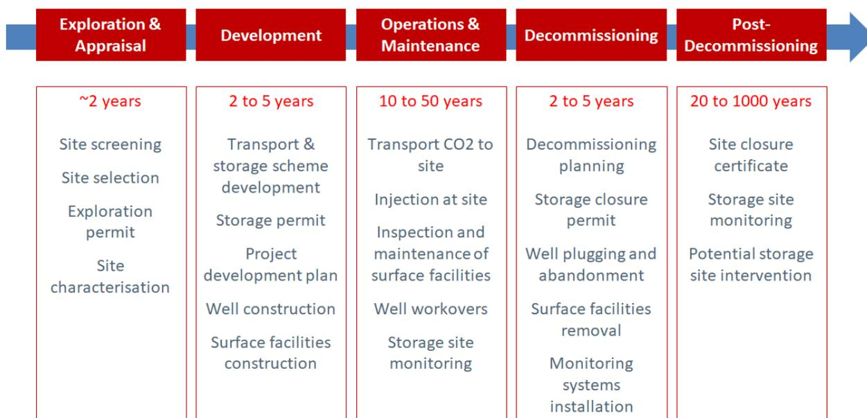
Figure 4.19: Indicative CCUS Project Lifecycle Stages
