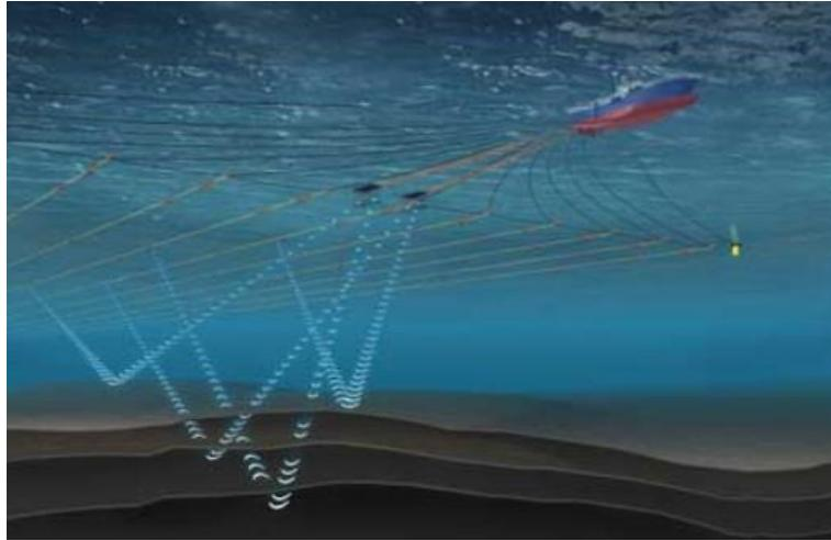
Figure 4.20: Typical "Towed Streamer" Seismic Survey Arrangement
