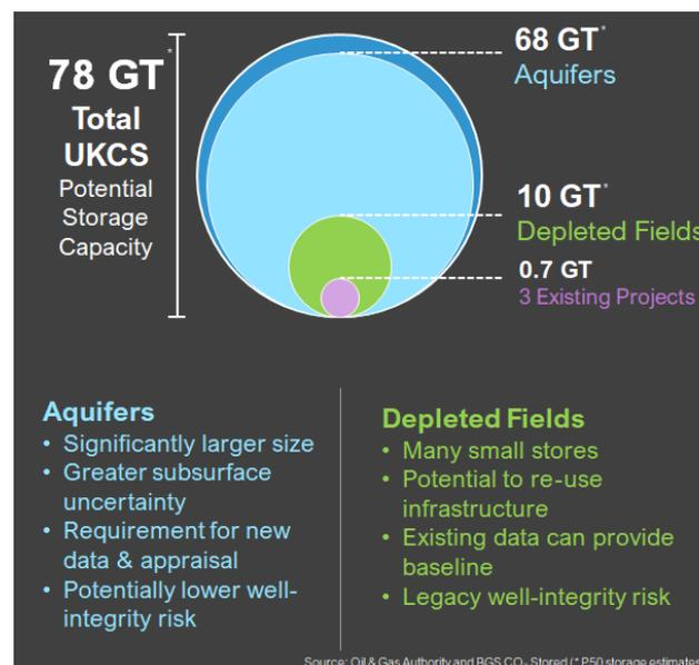
Figure 4.15: UK Offshore CO<sub>2</sub> Storage Potential for Main Types of Geological Storage [16]
