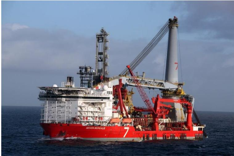
*Figure 4.21: Typical S-lay Pipeline Installation Vessel*
