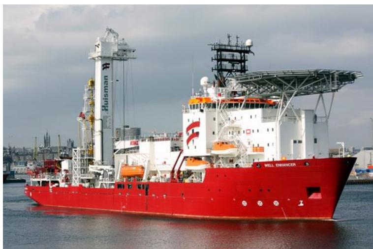
*Figure 4.28: Typical Light Well Intervention Vessel*
