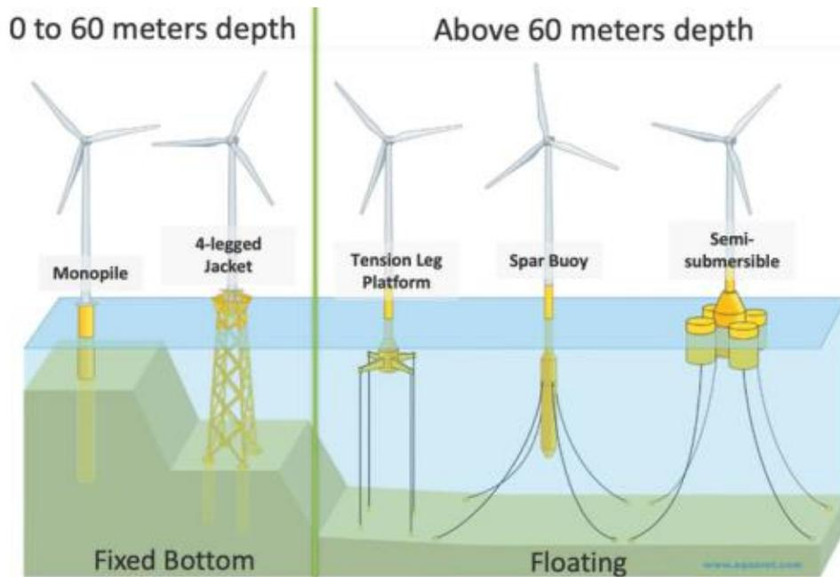
Figure 4.2: Fixed versus Floating Offshore Wind Substructures [9]
