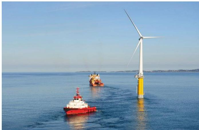
*Figure 4.11: Typical Operation to Tow Floating Wind Turbine to Site*
