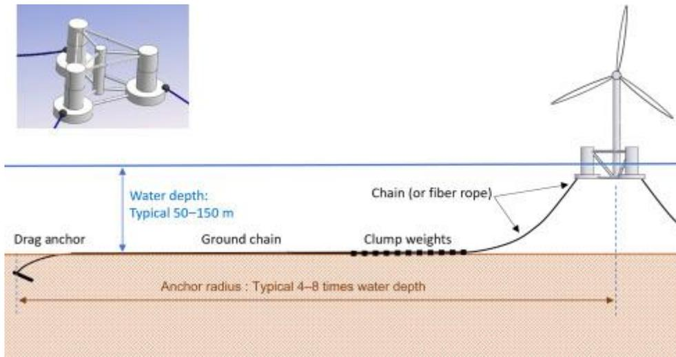
Figure 4.3: Typical Spread Mooring Design with Catenary Lines [13]
