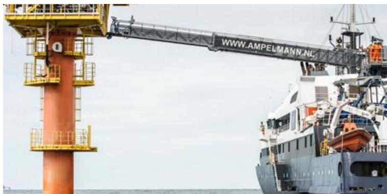
Figure 4.12: Typical Service Operation Vessel with Walk-to-Work Platform
