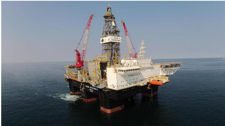
*Figure 4.23: Typical Semi-Submersible Drilling Rig*
