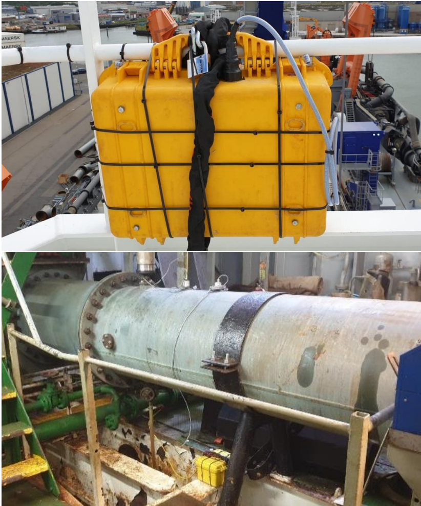
EMSc hardware – black box unit (top), sensor (bottom)
