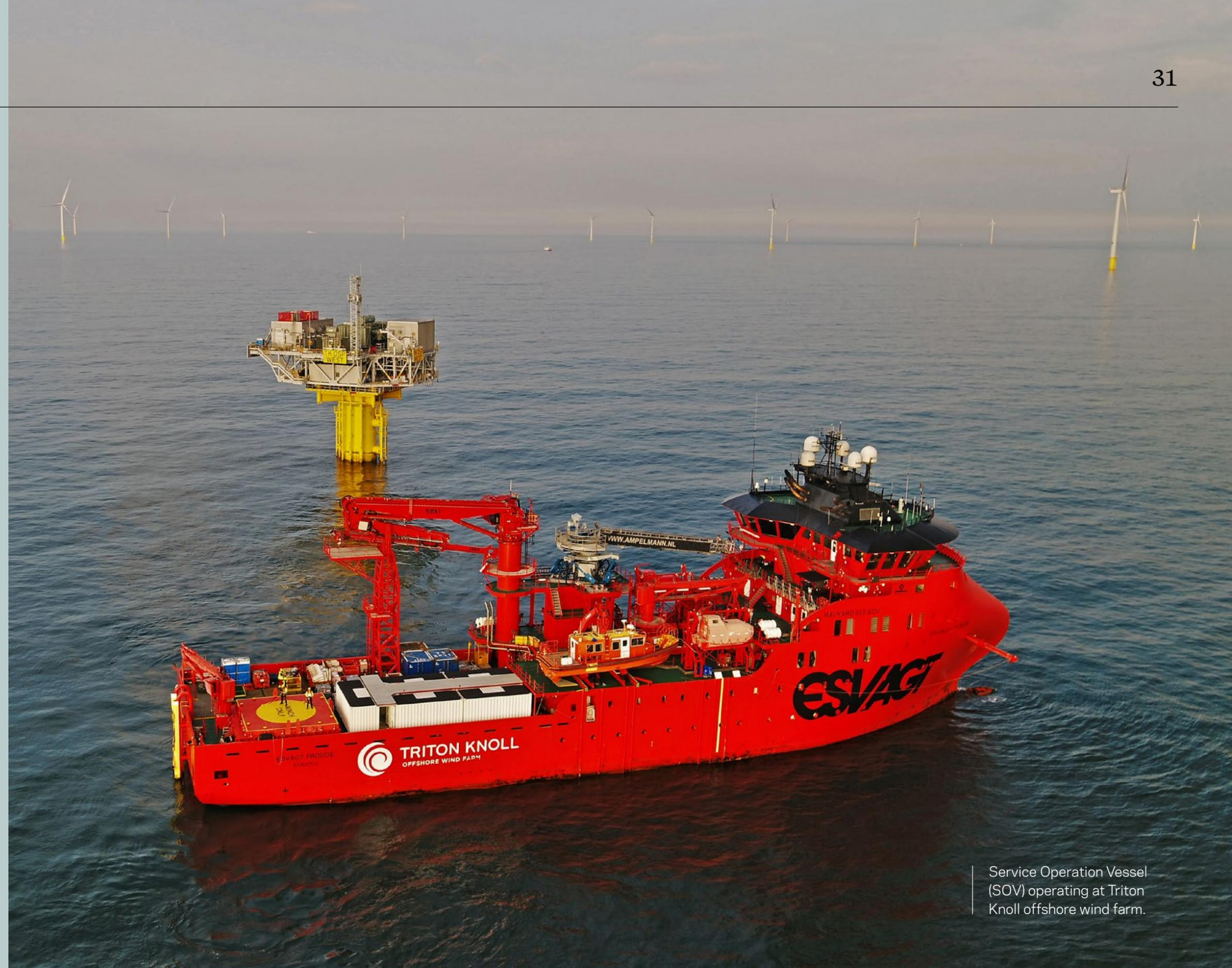
Service Operation Vessel (SOV) operating at Triton Knoll offshore wind farm.
